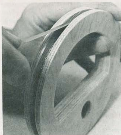
Fig. 9. Cover the coax shield braid with a single layer of plastic electrical tape.
