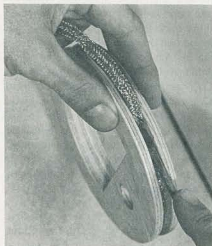
Fig. 7. The 20-turn coil is shielded with the braid from RG-8U coaxial cable.
