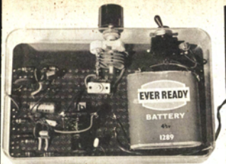
The complete detector unit ready for mounting on the handle and connecting to search coil
