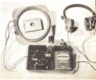
Top left—the search coil; top right—the headphones; bottom—the electronic detector
