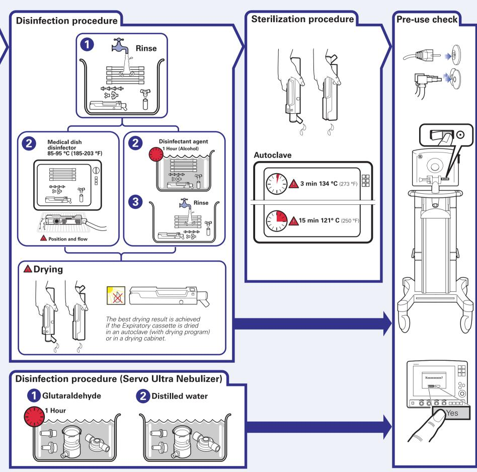
Servo<sup>f</sup> Ventilator System-Routine cleaning wall diagram V 1.0.0 Order No.: 65 15 014 E313E
