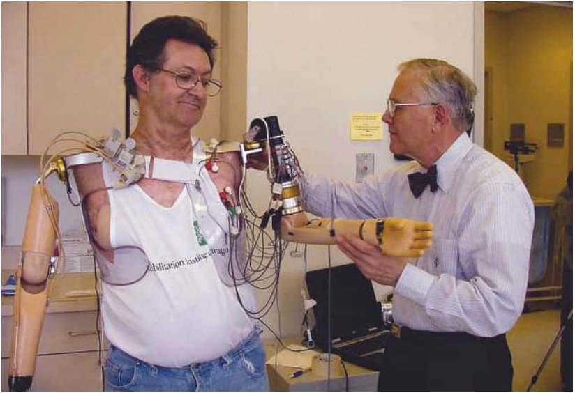
Figure 3 The advanced prosthetic device acting as Jesse Sullivan's left arm receives inputs rerouted from the nerves in his chest and the muscle activity that myoelectrode sensors detect (courtesy Rehabilitation Institute of Chicago).
