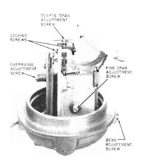
ZERO ADJUSTMENT - All output readings are moved up or down scale an equal amount by turning the zero adjustment screw.
