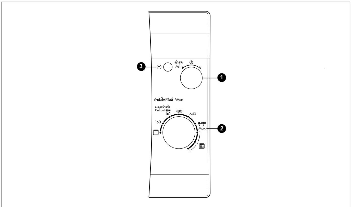
1. **TIMER / WEIGHT SELECTOR CONTROL:** Used to set the cooking time.
