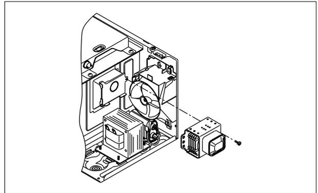
**CAUTION :** Never install the magnetron without the metallic gasket plate which is packed with each magnetron to prevent microwave leakage. Whenever repair work is carried out on magnetron, check the microwave leakage. It shall not exceed  $4\text{mW}/\text{cm}^2$  for a fully assembled oven with door normally closed.
