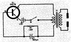
Unusual application of filament transformer steps up Q1's pulse output to excite the electrodes—and any one who happens to be holding on to them.
