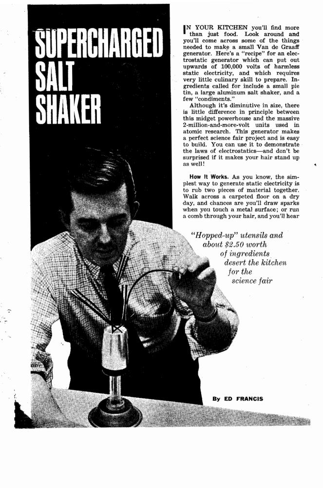
things snap, crackle, and pop. While this static electricity is commonplace, it is no different from that produced by the little Van de Graaff generator "cooked up" here. A hollow insulating column held in place by a pie-plate base supports a salt-shaker dome. Within the base, a small toy motor drives a rubber belt around a plastic pulley.
