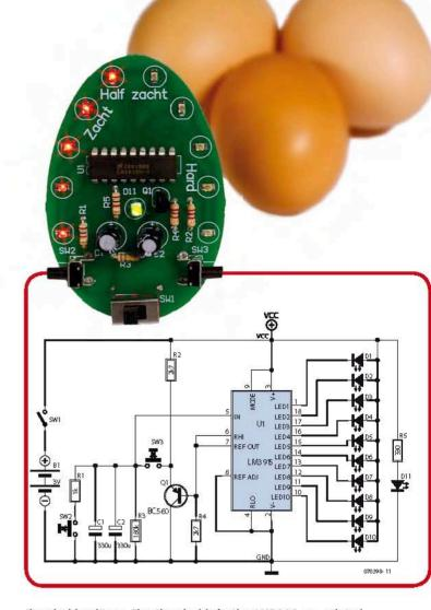
threshold voltage. The thresholds in the LM3915 are related exponentially so that they compensate for the discharge curve. The time period between each LED going out is now equal.
