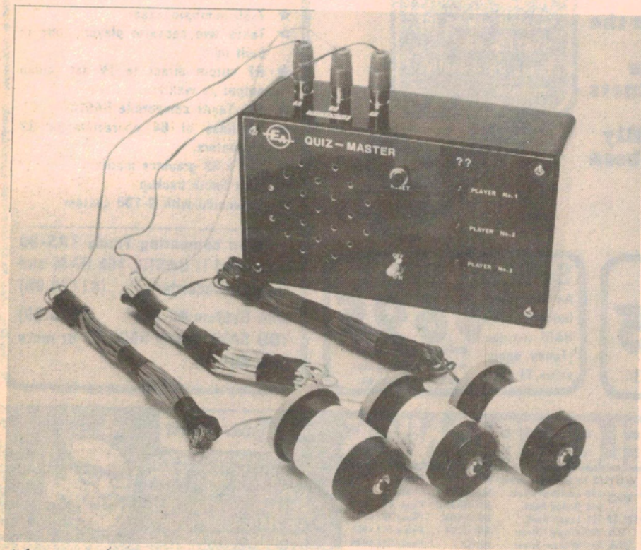
A front panel LED comes on to indicate which of the three buttons has been pressed first. Plastic film cannisters were used to house the player buttons.
