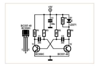
flows to C1 through R3, eventually allowing the voltage across the capacitor to rise high enough to open up T2 again. This, in turn, causes the right side of C2 to be pulled down by T2, which causes T1 to block all current, allowing C2 to be charged by R2 until T1 starts conducting again, leaving the cycle right where it started. This goes on for all eternity. Well, at least until the battery dies...
