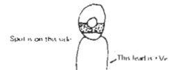
ABOVE: some tantalum capacitors are not marked with a "+" as in the photo. They instead have a dot on one side only.
