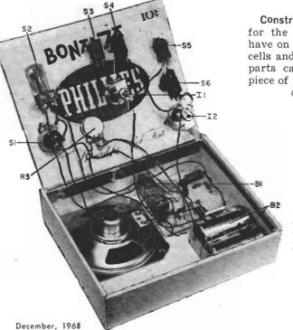
Construction. Many of the parts needed for the Gadget Box you will probably have on hand. Except for the speaker, D cells and holder, lamps, and controls, all parts can be mounted on a 3"-square piece of perforated board, using flea clips (Continued on page 109)
