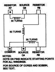
FIG. 5—TRANSFORMER T1 WINDING. This is the "footprint" for driver transformer T1. Drill two holes through the wooden frame member between the two compartments, and drill mating holes in the two insulating blocks. Drill a single hole in the opposite sides of each block and fasten the ladder strips to the blocks with screws, as shown in Fig. 3. Then attach the insulation
