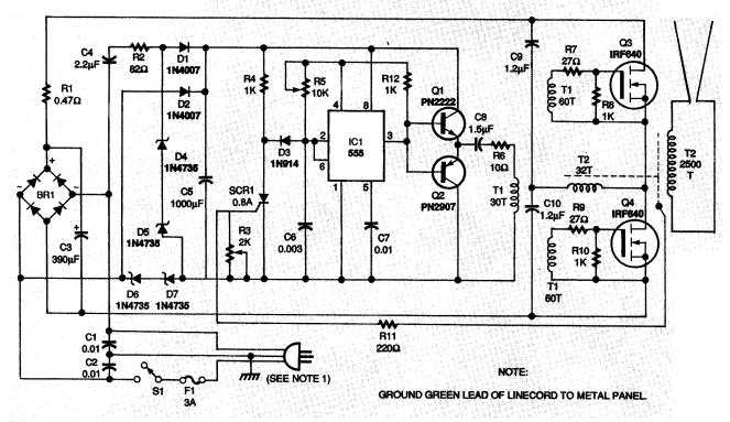
FIG. 1—SCHEMATIC FOR HIGH-VOLAGE power supply. All components except transformers are standard.
