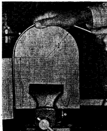
Fig. 3. Carefully bend the rod around the wood form to obtain a smooth shape in the loop. Rod must be clean and free from burrs to permit the ring to travel freely without interference.
