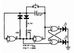
(Note that IC pin numbers in the diagram apply for both the 4001 and 4011.) With this circuit, it is necessary to adjust for a 50% clock duty cycle, using the potentiometer. If you don't have an oscilloscope to do this, simply measure the direct current flowing through each LED while adjusting the pot. When the same current level flows through each LED, the clock will be adjusted for a 50% duty cycle. —Ed Johnston, Oshawa, Ontario, Canada.
