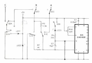
S2A, S2C and S2D open with respect to the power supply as shown, there is no input. How can the circuit work?
