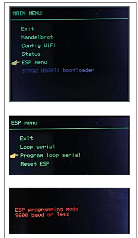
Figure 13. Configuring the Nucleo as a programming interface for the ESP8266 module.
