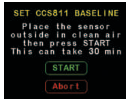
Screen3: this screen allows you to set the baseline (zero point) for the CCS811 sensor. Initially, this should be done once a week, but after a couple of months, the baseline will only need to be set once a month.
