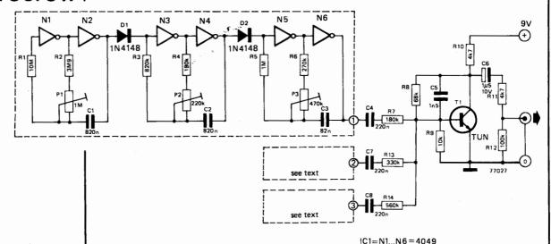
gates oscillator N3/N4, which in turn gates oscillator N5/N6. The result is that this last oscillator produces intermittent bursts of pulses, which makes the sound very realistic. The output can be taken from the righthand side of C4 and be fed to an audio amplifier and suitable (weatherproof) loud-
