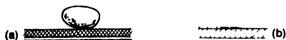
Fig. 1 (a): Solder on to non-metallic or unclean surface (b): Solder on to clean metallic surface
