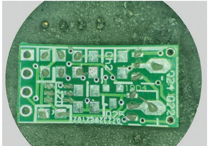
The board used during reflow test, showing solder paste applied to pads. The amount shown here is more than enough!
