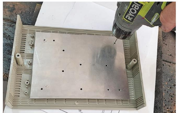
Once you've drilled out the baseplate (download the PDF from [siliconchip.com.au](http://siliconchip.com.au)) it can be used as a template for drilling the four required holes in the case (these align with four of the pillars moulded into the case).
