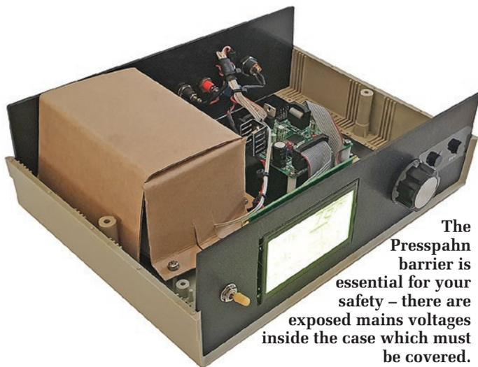
The Presspahn barrier is essential for your safety – there are exposed mains voltages inside the case which must be covered.
