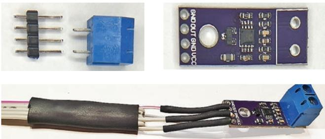
rather than eyelet lugs, but we feel that using a crimped connector makes it a bit tidier. Just make sure they are securely crimped. Apply insulation to all of these connections, and double-check them, then cable tie them all together, so that if one comes loose, it can't go anywhere.
