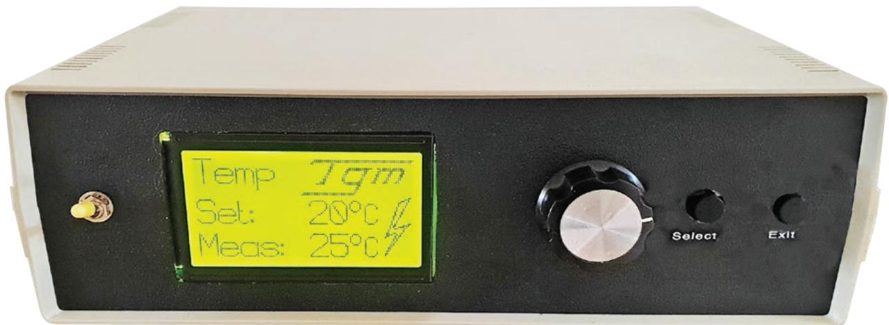
Four holes must be drilled in the front panel (follow the drilling diagrams on [siliconchip.com.au](http://siliconchip.com.au)) but there is also a cutout required for the display. We used a Dremel to cut out the rough hole then finished it off with a fine file. The same system can be used for the IEC mains socket cutout on the rear panel.
