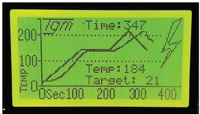
Reflow display showing target and actual temperature profiles.
