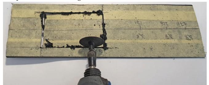
Covering the panel with masking tape before cutting out the display window has two benefits: (a) you can much more easily mark the position on the tape (along with other hole locations) and (b) it tends to make the waste stay in place, resulting in less mess!
