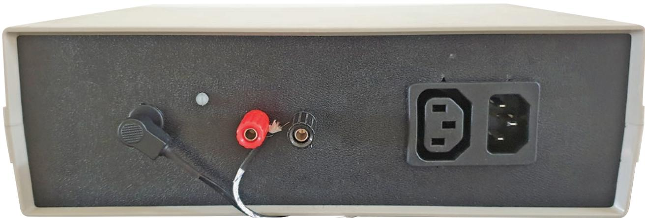
The rear panel sports the 9V DC input socket (left) with the polarised thermocouple terminals alongside. At the right end is the twin IEC mains output/input socket which is the raison d’être for this project: mains comes in to the right-hand (male) socket; controlled mains to the toaster oven comes out of the left-hand (female) socket.
