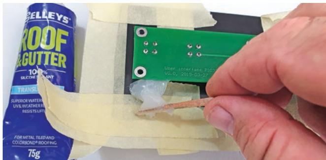
To avoid screw heads protruding from the front panel, we glued the LCD to the rear of the panel using silicone sealant. The masking tape showed us where the glue was to go.
