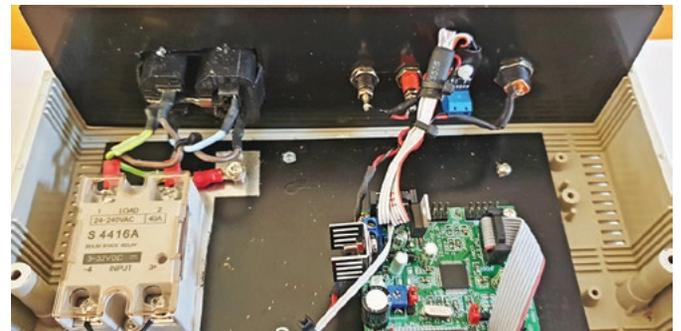
**A view of the rear panel connections – again, this is before the Presspahn insulation barrier is installed. Don't forget it!**
