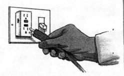
Use Ground Fault Circuit Interrupters.
