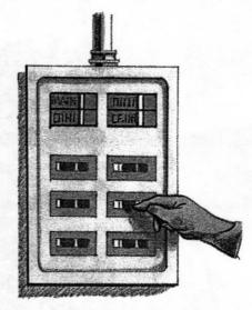
Switch off power at the fuse or circuit-breaker box, or pull the plug.
