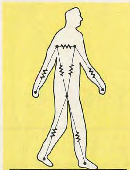
FIG. 1—A PERSON CAN be modeled as a network of resistances.
