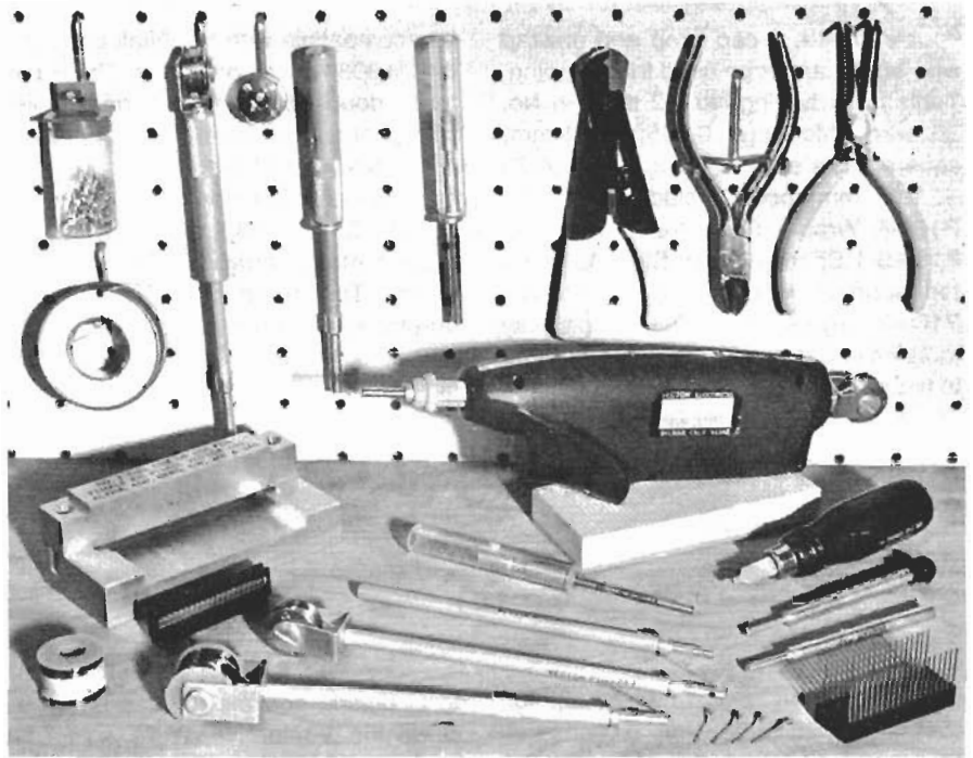
Typical Wire Wrap tools, including power wrapper.
