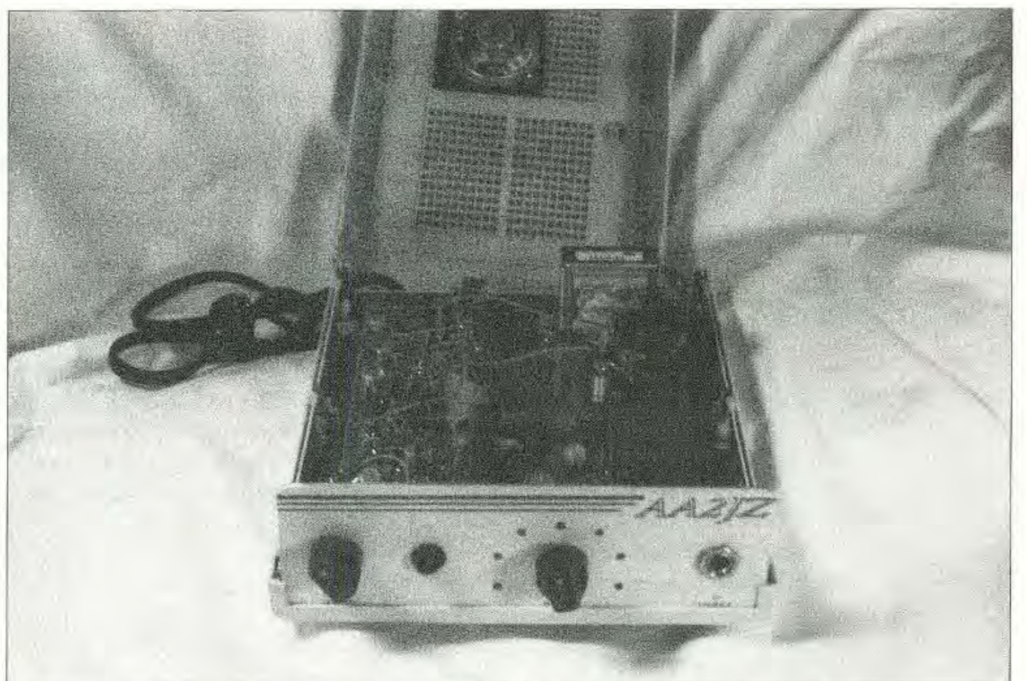
Photo B. The panel slips into slots and the top snaps over it all to keep it together.
