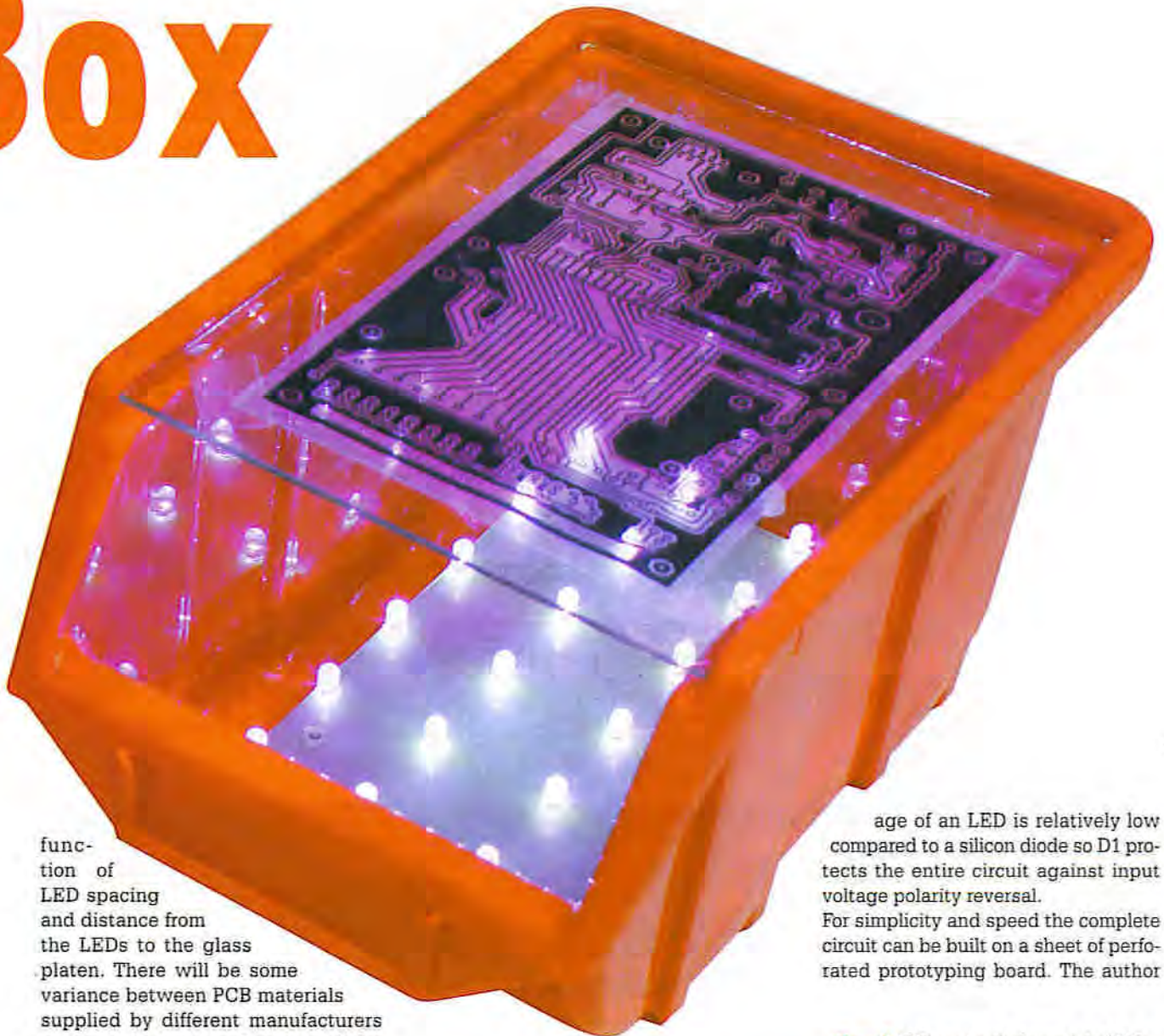
Figure 2. LED layout on the Eurocard sized PCB.
