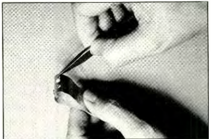
Fig. 6. Shown here is one way to get the release liner started. Use sharp-pointed tweezers for handling patterns.
