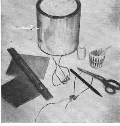
Except for epoxy resin compound and hardener (in can and small bottle at top), all materials used in circuit potting are common household items.
