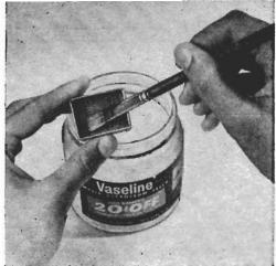
To prevent potting compound from adhering to form, liberally coat all interior surfaces of the form with Vaseline using a brush or a scrap stirrer.
