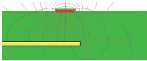
Figure 3: A trace routed too close to the edge of the board can produce EMI.
