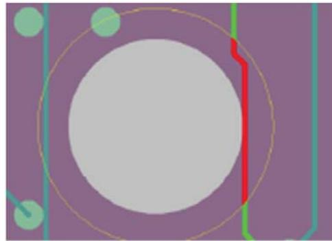
Figure 4: A trace routed near a large void on the reference plane can produce unwanted EMI.
