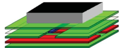
Figure 8: An IC mounted over a plane split.
