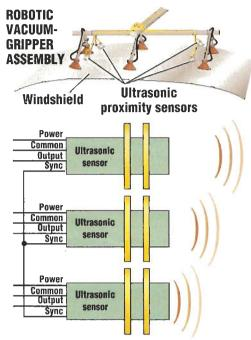
Four multiplexed ultrasonic proximity sensors detect the windshield angle for proper alignment of a robotic vacuum-gripper assembly. Multiplexing the ultrasonic bursts from each sensor prevents interference between sensors. Wiring the sync inputs of each sensor together as shown activates the multiplex feature.
