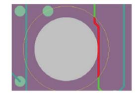
*Figure 4: A trace routed near a large void on the reference plane can produce unwanted EMI.*
