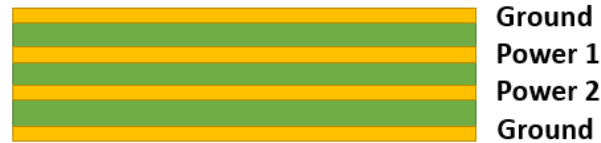
Example stackup for multiple power planes.
