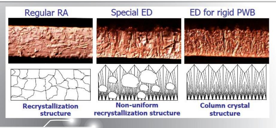
\*Comparison of crystal structure – crosssectional observation of cu. foil crystals after annealed
