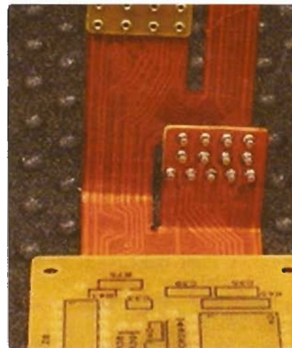
Conductors passing through a bend area should always run perpendicular to the bend as seen on the left, not at an angle as seen on the right.
