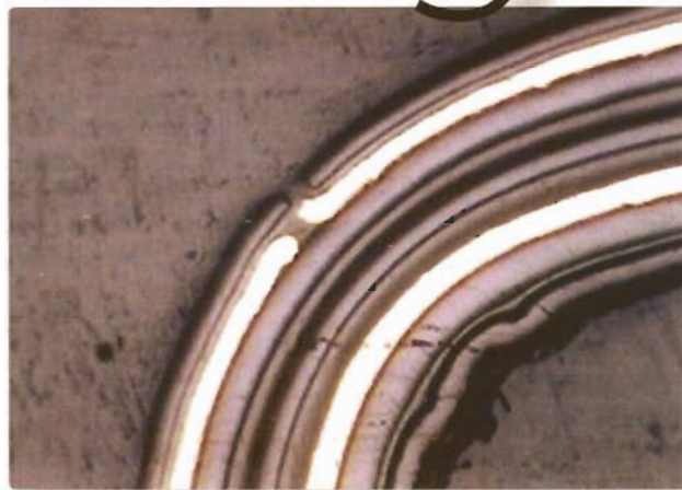
Improper design and handling can create tears and cracks in the outer layers and wrinkling or delamination of the inner layers.
