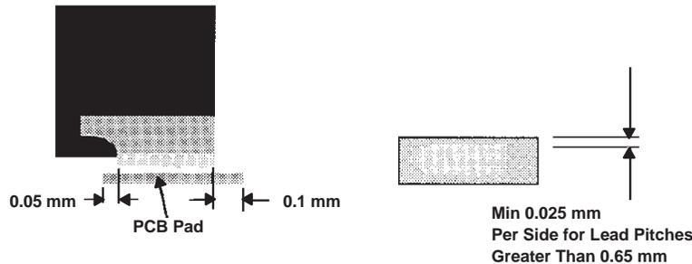
**Figure 3. Substrate/PCB Lead Finger Geometry**
