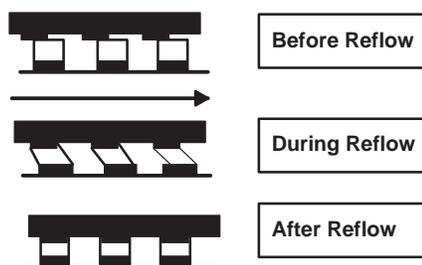
**Figure 7. Package Self-Alignment at Reflow**
