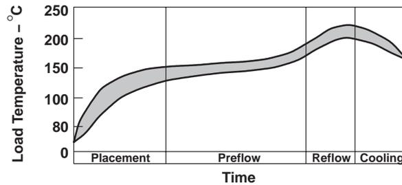
Figure 8. QFN/SON Load Temperature vs Reflow Profile
