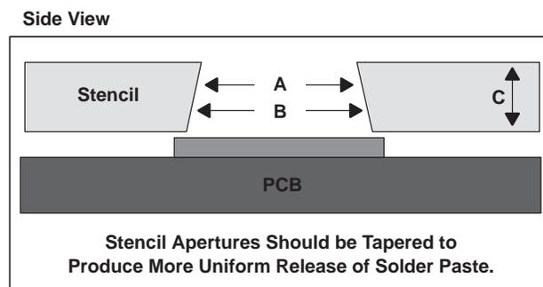
**Figure 5. Solder Stencil Profile**
