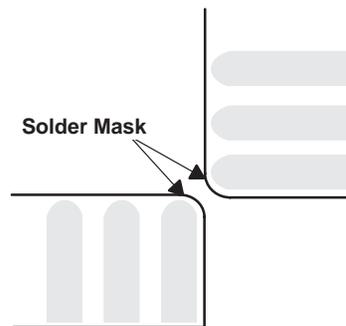
Figure 4. Substrate/PCB Solder Mask
