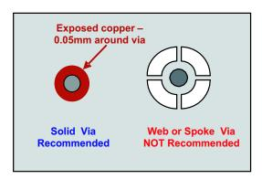
Figure 3. Via Connection at the bottom copper plane
