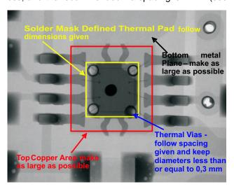
Figure 4. X-Ray - DGN Device
