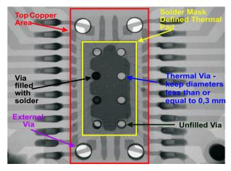
Figure 5. X-Ray - PCB Device With Internal and External Vias
