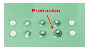
Figure 7. Protrusion at the Other Side of Board
