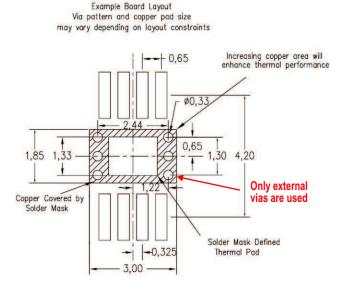
Figure 6. Example of Using Only External Vias
