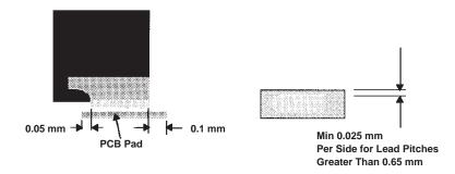
Figure 3. Substrate/PCB Lead Finger Geometry
