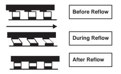
Figure 7. Package Self-Alignment at Reflow
