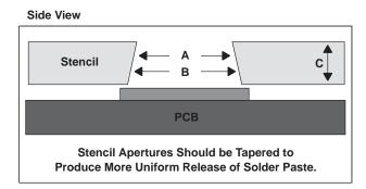
Figure 5. Solder Stencil Profile
