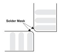
Figure 4. Substrate/PCB Solder Mask
