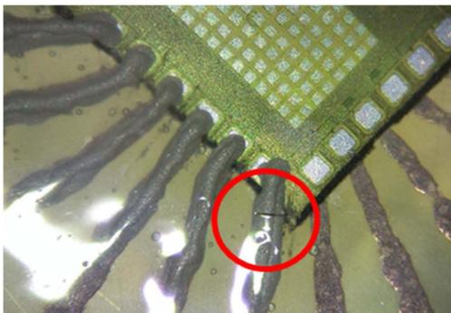
**Fig. 7: Crack in Printed Interconnects on VDD Line**
