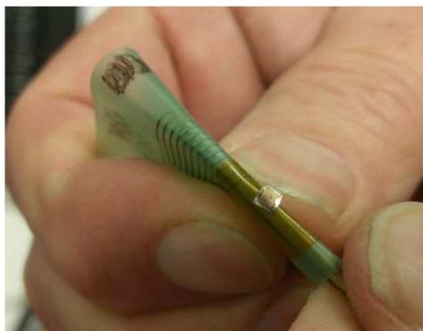
**Fig. 3: Substrate Failure at 2.5mm RoC**
