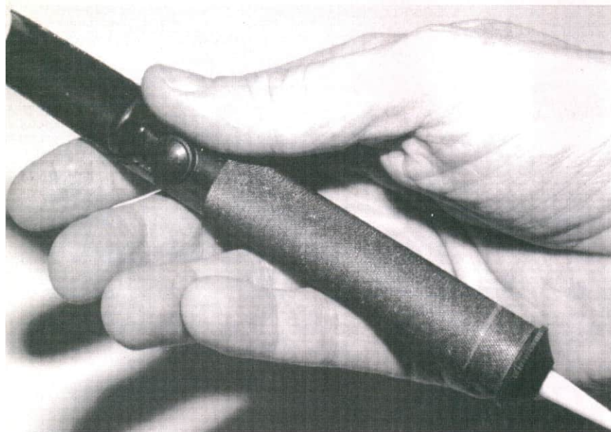
A typical solder pump; the nozzle is seen at the right and the release button is just below the thumb.
