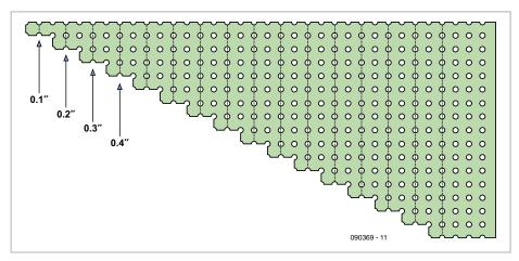
a piece of wire and fold it sharply around the indentations corresponding to the selected pitch. A neat wire link is the result, with exactly the right pitch and ready for soldering tightly into the PCB or prototyping board. With close-fitting wire links the board looks much better and they are also mounted much more quickly.
