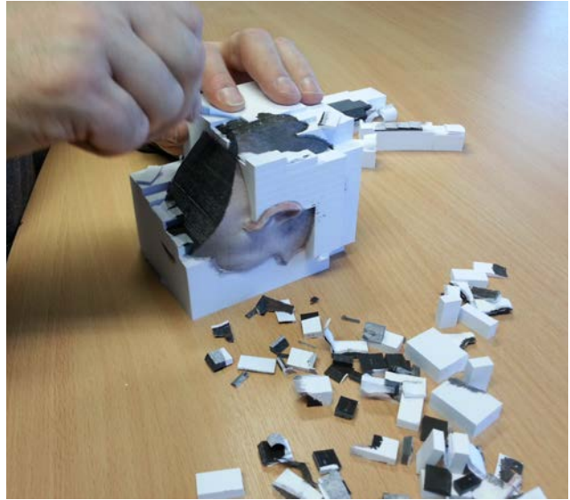
Fig. 4 Quickly and easily peel the supporting paper away from the part. This can be accomplished with your hands and ordinary tweezers; no need for chemicals. The head model emerges.
