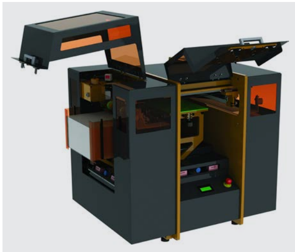
Fig. 7 Three reams of paper are placed in the paper feed door. Finished parts are removed from the front door.
