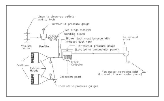
Figure 5-6. Exhaust system schematic.
