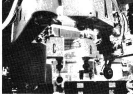
Scara robots in an IBM typewriter assembly facility each have four degrees of freedom.
