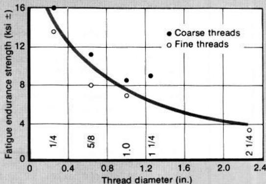
Fatigue endurance strength drops with increasing thread diameter, and is somewhat higher for coarse threads than for fine threads. Fasteners used in these tests had ultimate tensile stresses of 180 to 200 ksi, and were subjected to a mean static stress of 100 ksi. Values for fasteners with cut threads would be similar.
