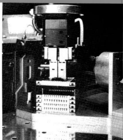
*Connector assembly uses Seiko RT 3000 robot to insert a series of wires. Only 12 seconds are required for the robot to select the proper wire, cut it, strip it, and secure it in its proper slot.*
