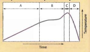
The typical CuproBraze temperature cycle calls for a slow heatup to let binder in the brazing paste burn off (A). The heat-exchanger core and fixture are allowed to equalize at around 550°C before brazing begins (B). The brazing period begins when the brazing powder reaches 600°C. Here, the filler metal wets and alloys with the base metal (C). Cooldown should be 1°C/sec or slower to 550°C to prevent thermal distortion (D).
