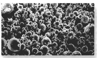
fine-grained spheres in a nitrogen atmosphere. The average particle size is 15 to 30  $\mu m$  with particles over 90  $\mu m$  sieved out. OKC600 is only available as powder, which can be mixed into brazing-pastes.
