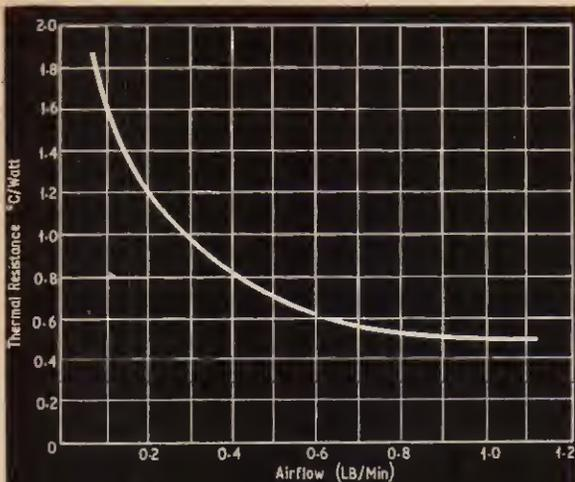
Fig. 6. Heat sink performance with forced airflow
