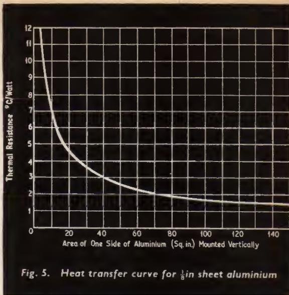
Fig. 5. Heat transfer curve for  $\frac{1}{8}$ in sheet aluminium
