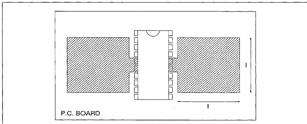
Figure 8 -  $R_{th(j-a)}$  of POWER DIP 16+2+2 vs side l for heat sink on the PCB lower side
