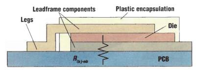
A single, simple conduction path from device junction to package mounting base.
