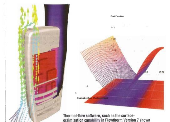
It's no secret that the mobile-device market is the primary driver of innovation within the electronics industry. But the small size of modern mobile devices also creates thermal-management challenges. Cramped corners in mobile devices reduce internal airflow and lower the maximum allowed external temperature.
