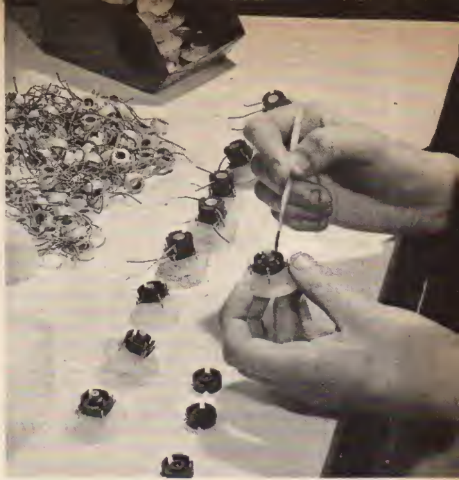
Pye of Cambridge use epoxy adhesives to bond the two halves of ferrite pot cores for telephone equipment
